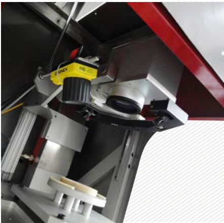
XL-Box marking station with deported reading system
